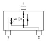
This transistor is a electrostatic sensitive device. Please handle with caution.
